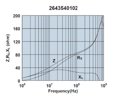
Impedance, reactance, and resistance vs. frequency.
