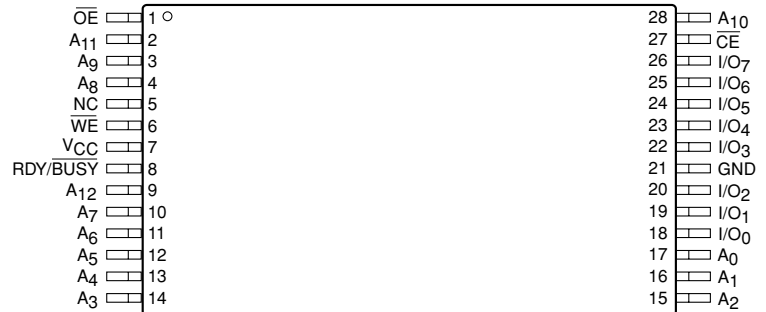
TSOP Package (8mm x 13.4mm) (T13, H13)
