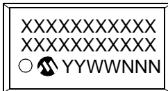
14-Lead SOIC (3.90 mm)
