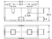
Note: The Cover has six thin, easy-to-separate portions for easy lead wire connections.
