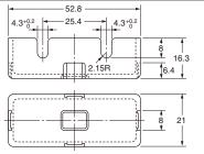
Note: The Cover has five thin, easy-to-separate portions for easy lead wire connections.
