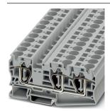
Feed-through terminal block, nom. voltage: 1000 V, nominal current: 76 A, connection method: Spring-cage connection, number of connections: 3, cross section: 0.2 mm² - 25 mm², AWG: 24 - 4, width: 12.2 mm, color: gray, mounting type: NS 35/15, NS 35/7,5
