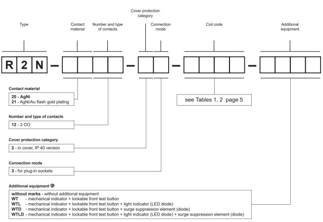
(3) T - orange colour (AC coils), green (DC coils). WT - standard equipment of relays. WTD, WTLD - available only in relays with DC coils.
