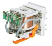
Application of electronics made in the SMD technology: additional equipment L (LED diode) and D (diode) are located on the printed circuit board; the change of the position of the LED diode and optimization of the quality and intensity of its light provide certainty that the relay is in operation status when the LED is on.
