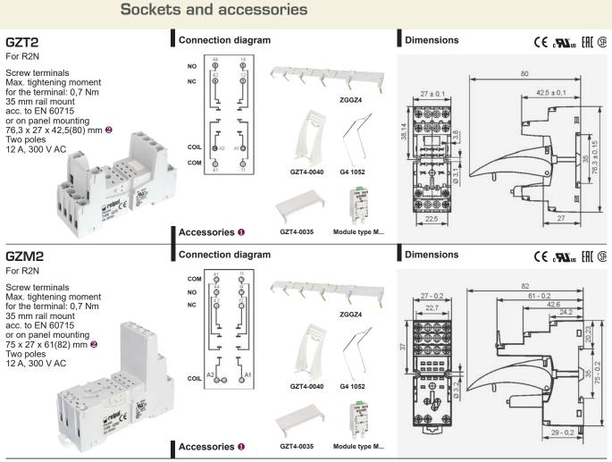
Mounting and sub-assemblies of accessories in the socket - see page 9. Signalling / protecting modules type M... - see page 12.
