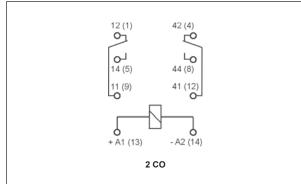
Note: the indicated polarization of the supply refers to the relays with extra equipment  ${\bf D}$  - surge suppression element (diode) - for DC coils only.
