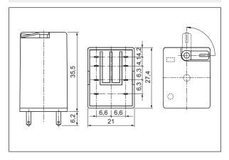
**Dimensions** - plug-in version, with test button (no latching) or with plug (no manual operation)
