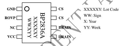
Figure 2. Pin configuration
