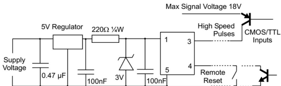
Mount the 100nF (transient suppression) capacitor as close to the unit as possible.
