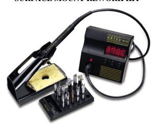
The Antex surface mount rework station is an entry level station which gives the user the ability to remove most component types without damage to the circuit board or surrounding components. Each rework tool is heated to the exact temperature required by the component by means of a microprocessor control inside the soldering station.
