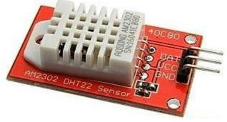
Voltage: 5V; Temperature:  $-40^80$ 'C, +/0.5'C; Humidity:  $20^90$ %RH, +/-2%RH; Suitable for Arduino, SCM; A product for Arduino that works with official Arduino boards.
