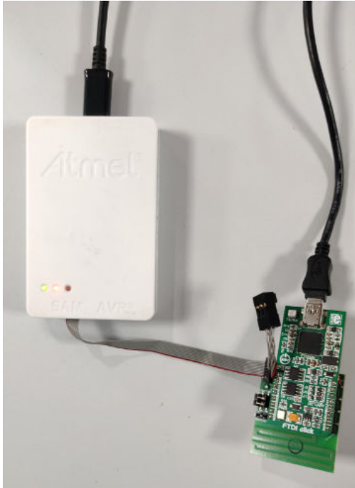
Figure 4-11. Connecting Programmer/Debugger with ATSAMR30M Sensor Board
