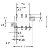
**Terminal Arrangement and Internal Connections** (Top View)
