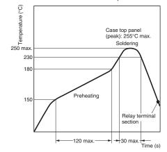
3. The thickness of cream solder to be applied should be between 200 and 250 μm and the land pattern should be based on Omron's recommended PCB pattern. To maintain the correct soldering joint shown in the following diagram, we recommend applying solder using the soldering conditions shown above. Check the soldering in the actual mounting conditions prior to use.
