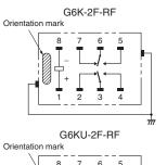
Note: Check carefully the coil polarity of the relay
