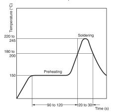
2. Temperature Profile for Lead-free Solder (Measured at the PCB)
