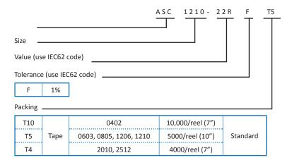
Note: For zero ohm jumper, substitute value and tolerance with the code R000
