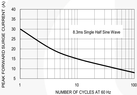
Figure 3. Maximum Non-Repetitive Forward Surge Current
