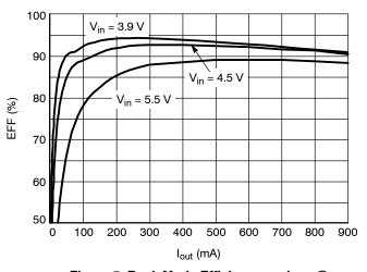
Figure 5. Buck Mode Efficiency vs.  $I_{OUT}$  @  $V_{OUT}$  = 3.1 V L = TDK RLF7030T-4R7
