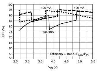
Figure 4. Efficiency vs.  $V_{IN}$  LED = Lumileds LUXEON III, L = TDK RLF7030T-4R7
