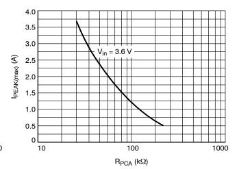
Figure 8. I<sub>PEAK MAX</sub> vs. R<sub>PCA</sub>
