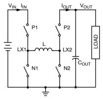
Figure 16. Basic Power Switches Topology
