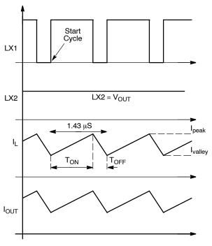
Figure 18. Basic DC-DC Buck Operation
