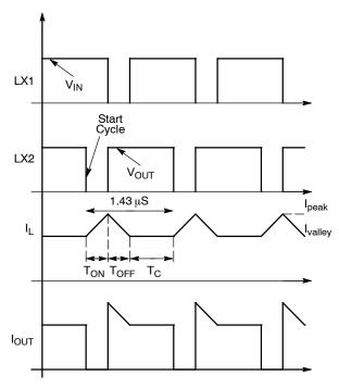
Figure 20. Basic DC-DC BB Operation
