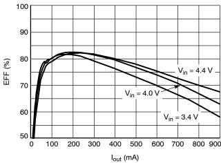
Figure 6. Buck-Boost Mode Eff. vs. I<sub>OUT</sub> @ V<sub>OUT</sub> = 3.8 V L = TDK RLF7030T-4R7
