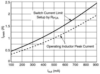
Figure 23. Inductor Peak Currents Vs. I<sub>OUT</sub> (mA)
