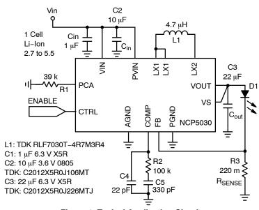
Figure 1. Typical Application Circuit
