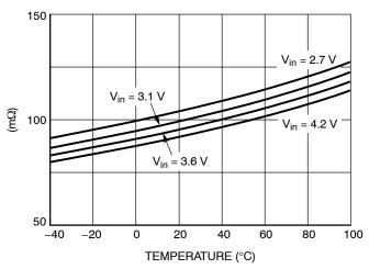
Figure 9. NMOS R<sub>DSON</sub> vs. Temperature
