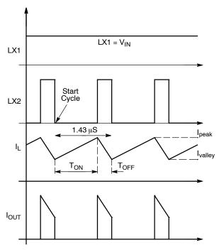
Figure 19. Basic DC-DC Boost Operation
