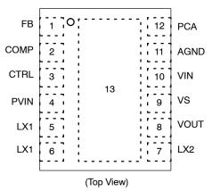
Exposed pad (Pin 13) is PGND must be soldered to PCB GND plane
