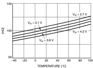
Figure 10. PMOS R<sub>DSON</sub> vs. Temperature
