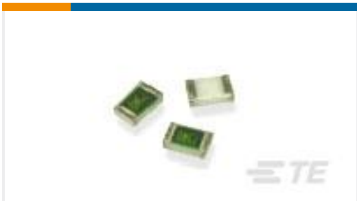
TE Part #1676197-2 RN 0805 15K4 0.1% 10PPM 1KRL
