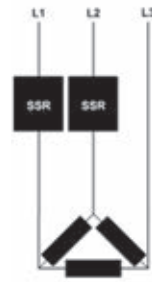
Two-phase SSR SOB to control heaters connected in delta (for high voltage, balanced or unbalanced loads)
