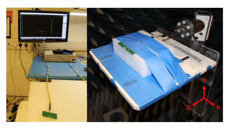
Figure 1. Impedance measurements (left hand) and peak gain, average gain, efficiency, and radiation pattern measurements (right hand).
