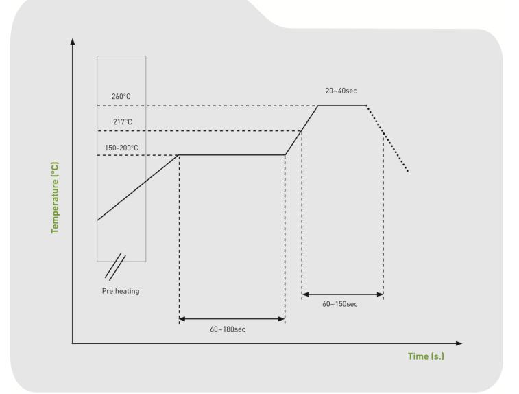
Figure 11. Reflow Temperature Recommendation
