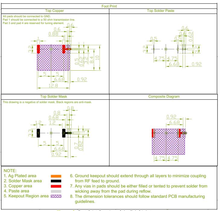
Figure 8. Foot Print Drawing of the ILA.01 Antenna
