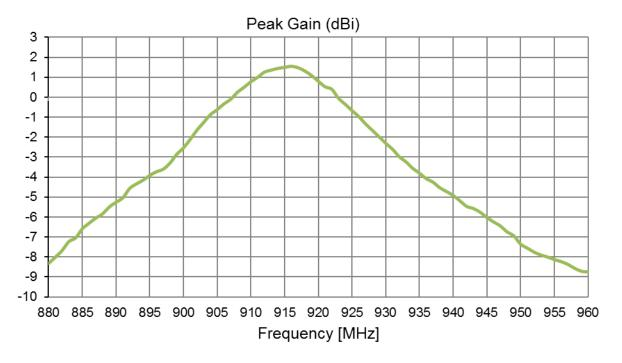
Figure 5. Peak Gain of 915 MHz ISM Band Antenna ILA.01
