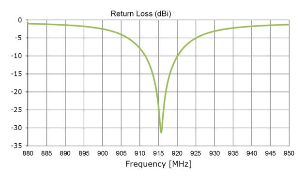
Figure 2. Return loss of 915MHz ISM Band Antenna ILA.01
