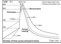
Wave Soldering (Flow Soldering)
