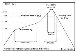
**IR Reflow Soldering**
