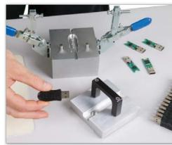
To overmould components using the Overtec system, first open the mould set and place the component inside. Next, load an **Overtec 5 FR** resin stick into an appropriate applicator, like the **Overtec 820-15**, switch on and allow it to reach operating temperature.
