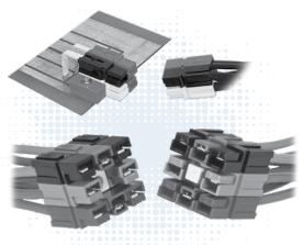
PP15-45 series are the smallest Powerpole® housings. They can be used for wire-to-wire or wire-to-board applications. Wire sizes from #20 AWG (0.75 mm²) to #10 (6 mm²) offer power capabilities up to 55 amps per pole. Finger proof housings and the ability to incorporate first-mate last-break ground connectors enhance the capabilities of this Powerpole® series.
