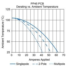
NOTE: PP25 PCB charts based on 0.002 in<sup>2</sup> foil on board side, mated to #12 AWG conductor on wire side. PP45 PCB charts based on #10 AWG equivalent copper foil on board side, mated to #10 AWG conductor on wire side.
