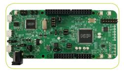
The MC56F83000-EVK is an ultralow-cost development platform for the MC56F83xxx DSC family allowing rapid prototyping and application development.
