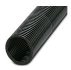
Protective hose, material: PA 6, UV-resistant: yes, flexible, degree of protection: IP68, color: black, flammability rating in acc. with UL 94: HB, inner diameter: 36 mm, Total length: 25 m
