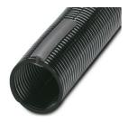
Protective hose, material: PA, UV-resistant: yes, flexible, degree of protection: IP40, color: black, flammability rating in acc. with UL 94: HB, inner diameter: 36 mm, Total length: 10 m
