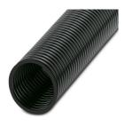
Protective hose, material: PA 6, UV-resistant: yes, flexible, degree of protection: IP68, color: black, flammability rating in acc. with UL 94: V0, inner diameter: 36 mm, Total length: 25 m
