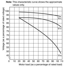
Note: For phase loss of phase R. Vst, Vtr, and Vrs indicate the motor terminal voltage at phase loss.
