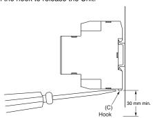
Leave at least 30 mm of space between the product and other devices to allow easy installation and removal.
