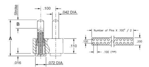
**Description:** Interconnect SLC Header Spring-Loaded Header Vertical Mount SMT Double Row Surface Mount **Plating Code:** Shell Plating:
