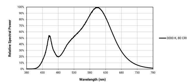
The following graph is the result of a series of pulsed measurements at 1400 mA and T<sub>1</sub> = 85 °C.
