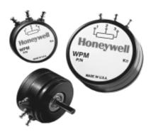
Available in servo mount styles, the WPM Series rotary transducer provides long life by utilizing the proprietary MystR® conductive plastic film, precious metal wipers and shielded ball bearings on the stainless steel shaft.
