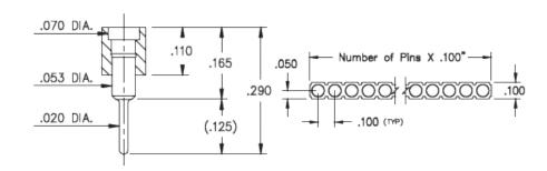
**Description:** Interconnect Flat Face Target Connector Spring-Loaded Header Vertical Mount Through Hole Target Single Row Through Hole
