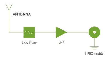
The AP.25E has a SAW filter on the front of it. The main use of the AP.25E would be for small devices where the GSM transmitter is close to the GPS/GALILEO antenna, it helps avoid burn-out of the LNA or the module due to interference from the GSM transmitter at out band frequencies.
