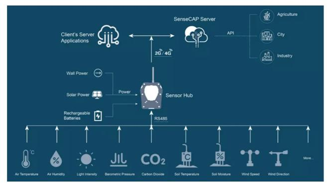
(SenseCAP Sensor Hub system architecture)
