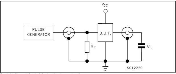
$C_L$  =15/50pF or equivalent (includes jig and probe capacitance)  $R_T$  =  $Z_{OUT}$  of pulse generator (typically 50 $\Omega$ )
