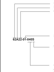
Style: A = 1/2" package, 5.0 Vdc Input, D = high torque w/5.0 Vdc input, V = 3.3 Vdc input Angle of Throw:
