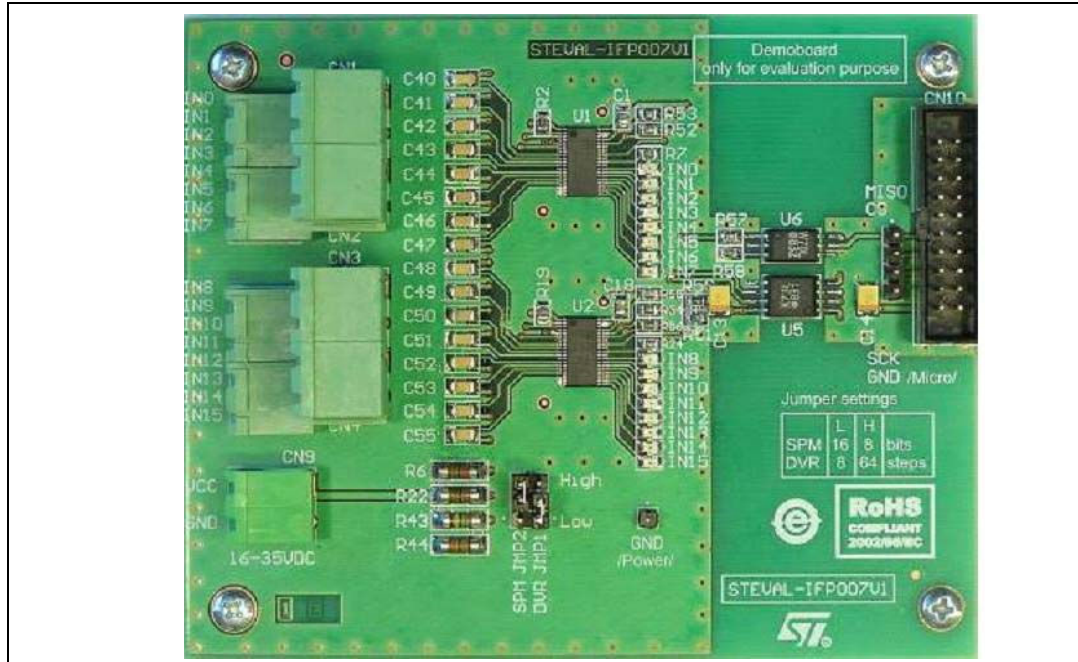
Figure 6. 8/16 input channel current limiter based on SCLT3-8, STEVAL-IFP007V1
