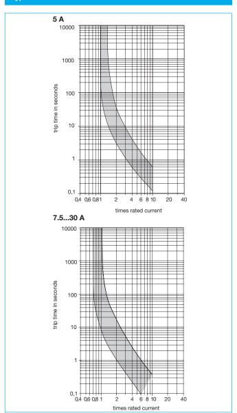
The time/current characteristic curve depends on the ambient temperature prevailing. In order to eliminate nuisance tripping, please multiply the circuit breaker current ratings by the derating factor shown below. See also
