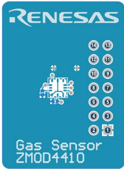
Figure 10. Sensor Board Layout – Top Layer with PIN Configuration on Connector X1
