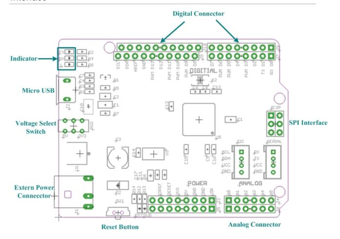
**U1:** 78M05 IC, Three-terminal positive voltage regulator.
