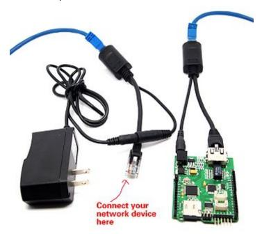
Method 2: Use separate power cable and Ethernet cable.
