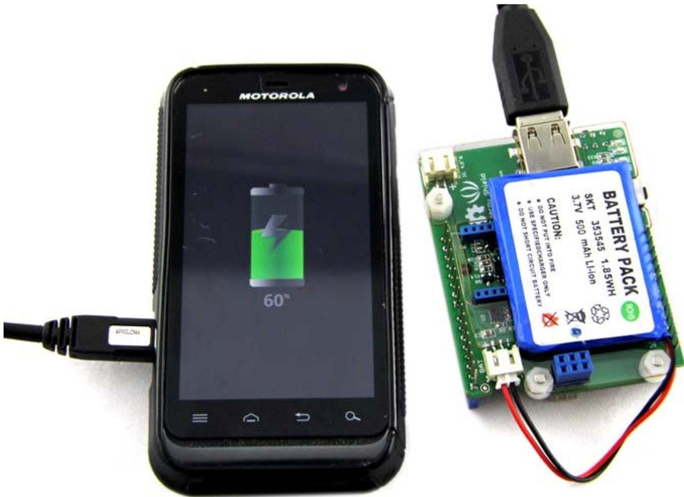
Use the standard USB port on the shield to supply power to mobile devices.
