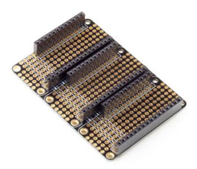
Perfect for any prototyping project, the Tripler provides space to add-on up to two FeatherWing accessories without any stacking header needs. Compatible with the newest generation of Particle developer kits (Particle Mesh).
