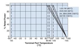
For resistors operated at a terminal part temperature of described for each size or above, a power rating shall be derated in accordance with the above derating curve. Please refer to "Introduction of the derating curve based on the terminal part temperature" in the beginning of our catalog before use.
