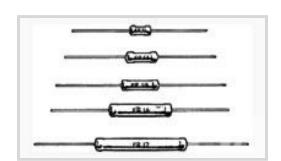
Resistor Type: Power Resistor
