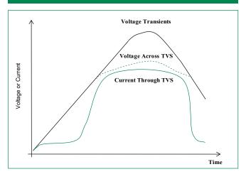
Figure 2 - Peak Pulse Power Rating
