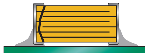
Type B: Fracture from top of device to bottom of device.
