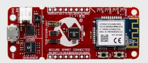
AVR-IoT WG Development Board (AC164160) PIC-IoT WG Development Board (AC164164)
