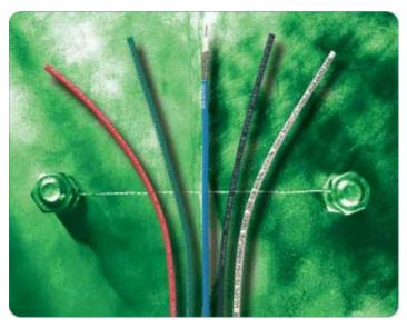
Van Damme plasma grade miniature video cable has been specifically designed to provide the best 75 Ohm performance possible for a small diameter video cable. It is mechanically based on RG179 and uses this BNC crimp type for robust terminations. It is ideal for rackwiring and multipin breakouts where a small overall diameter is essential, and is available in the 5 common colours most associated with video signals.
