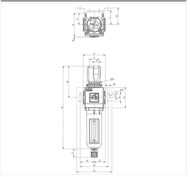
To remove the reservoir, allow a clearance of 60 mm from the bottom of the reservoir drain.
