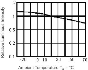
Luminous Intensity vs. Ambient Temperature
