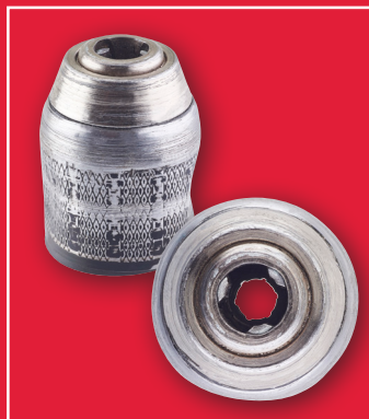
Broken chuck due to misuse
