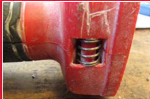
Spring assembled externally, proving unauthorised opening of tool
