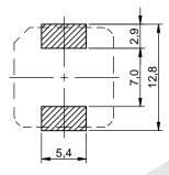
no sensitive traces underneath the component
