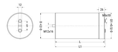
General Information Series C44U-M Dielectric Metallized Polypropylene Style DC Filtering, Energy Storage Features RoHS With Exemptions **REACH** SVHC (Pb - CAS 7439-92-1) SCIP Number cc1c1ec4-db9e-4815-b26b-e8a34ddfb776 Screw Terminals M6 Lead AEC-Q200 Nο Component 1020 g Weight Thermal Resistance = 5.8 C/W. Weight = 5100 Miscellaneous grams.
